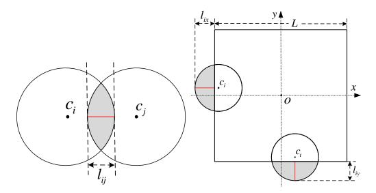
(a) Overlapping depth  $l_{ij}$  between two circles (b) Two kinds of overlapping depths between  $c_i$  and  $c_j$  a circle and the border of container
