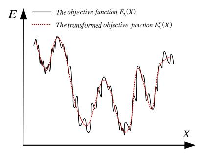
Figure 2 A schematic diagram illustrating the effects of the sequential random perturbation in the onedimensional case. The black line is the original potential energy surface  $E_L(X)$  of the objective function and the red dotted line represents the surface ( $E_L^P(X)$ ) transformed by the SRP perturbation operator. Note that the transformation of potential energy surface does not change the global optimum solution of the problem.
