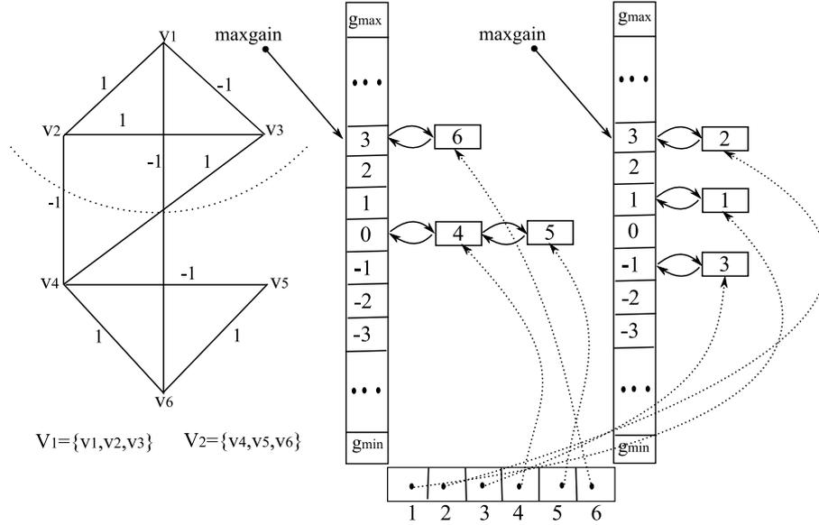
Fig. 1. An illustrative example of the bucket sorting data structure on a graph with 6 vertices
